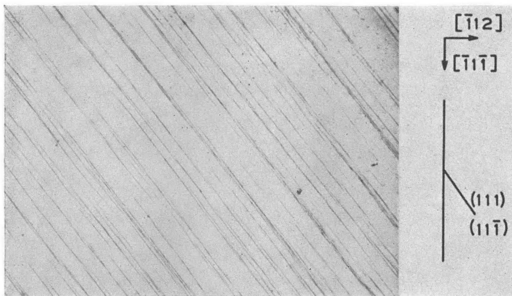
FIG. 8. Top surface of (110)[ \bar{1}12 ] Permalloy crystal after 50.5% thickness reduction, electropolished, and then further deformed lightly. No constraint on \epsilon_{y_2} . Slip plane traces consistent with predicted -a_2 , (111)[ \bar{1}01 ], and b_2 , (111)[011] slips. \times 140
