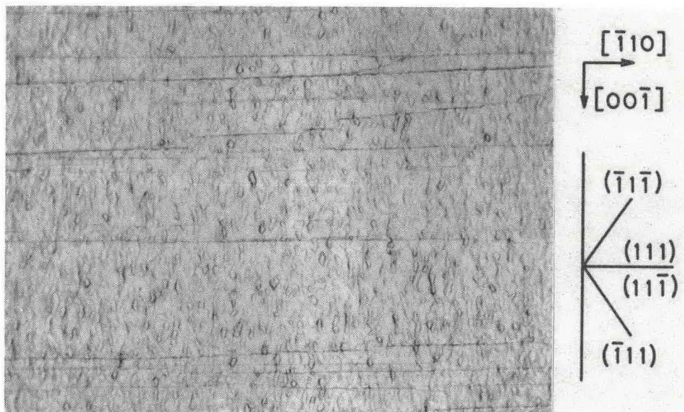
FIG. 7. Top surface of (110)[ \bar{1}10 ] aluminum crystal after 24% thickness reduction, showing absence of deformation bands. Slip plane traces are noted in margin. \times 280
